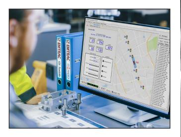
Workstation monitors can display current phase states for all equipped intersections, as well as a wide range of detection-input and vehicle activity. This activity may be displayed on a single workstation monitor—or it may be apportioned for display across a video wall.
